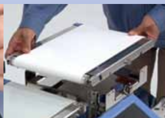
Replacing a conveyor
