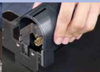
Replacing a gear motor
