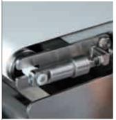
A simple, robust, automatic conveyor belt tensioning and tracking system maximises uptime. Once set, the system will automatically compensate for belt wear and lateral forces. The innovative design facilitates quick release of the tensioning roller to assist in rapid strip-down.
