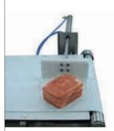
Automatic reject devices are available to suit most product inspection applications. These systems provide fast and efficient removal of contaminated product without the need to stop the production line providing enhanced levels of contaminated product control.
