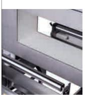
The combination of a fully welded "open design" conveyor frame with a search head free of dirt traps supports HACCP compliance. All contact parts are made from food quality materials ensuring there is no potential for product contamination.
